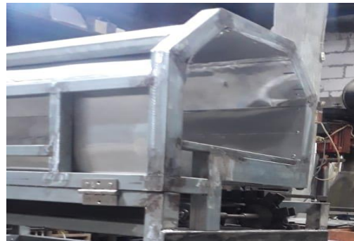
Gambar 3.22 Lapisan Dinding Gaswols.
